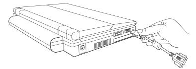
Sample connecting the Toshiba Mini RGB Adapter to the RGB (monitor) adapter port
